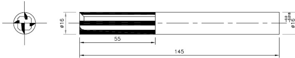
Fig.8 Reverse Taper profile (Carbide brazed) end mill
